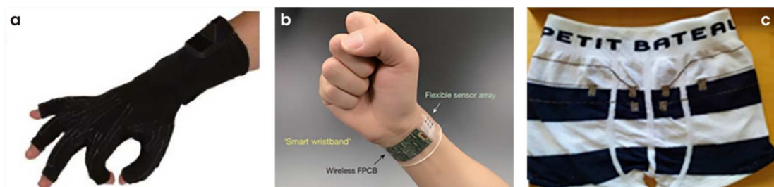
Figure 7. (a) DataGlove™ VRLOGIC with flex sensors [21]. (b) Photograph of a wearable FISA on a subject's wrist [45] (Reprinted with permission from Ref. [45]. Copyright 2021 Nature). (c) Trunk integrating leakage sensor embedded into children's underwear to detect urine leakage [46].
