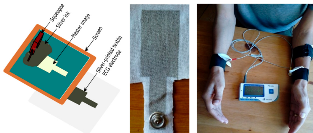
Figure 12. (Left to right) Block diagram for screen printing process; front view of the developed electrode; component placement setup for ECG measurement [74].
