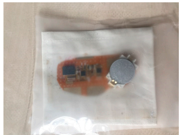
Figure 2. (a) Accelerometer diagram. (b) An accelerometer is sealed in an airtight envelope. PCB: printed circuit board.
