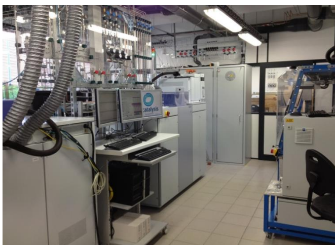
Fig. 3. Flowrence catalytic unit in the RealCat high-throughput experimentation platform in Lille.
